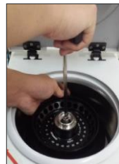
Tool for rotor without nut
