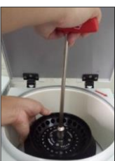
Tool for rotor with nut
