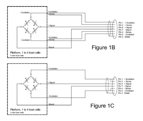
Figure 1B shows a preferred method to attach a 4 wire load cell, using a 6 conductor cable to go from the indicator to the platform or load cell where it connects to the 4 wires from the load cells. The Excitation and sense wires are connected together near the load cell.
