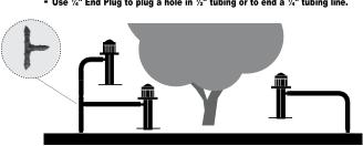
Note: Insert a 1/4" tee to use multiple sprinklers in one area. The use of multiple sprinklers is ideal for trees and plants that need additional watering.
