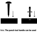
to insert a coupling into the distribution tubing. Place the coupling in the hole on the blunt end of the tool and push the exposed end into the distribution tubing.
