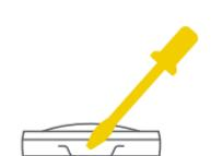
Sensors include one Lithium CR2032 battery. Annual battery replacement is recommended for optimal performance. See the "Replacing the Battery" section for instructions.
