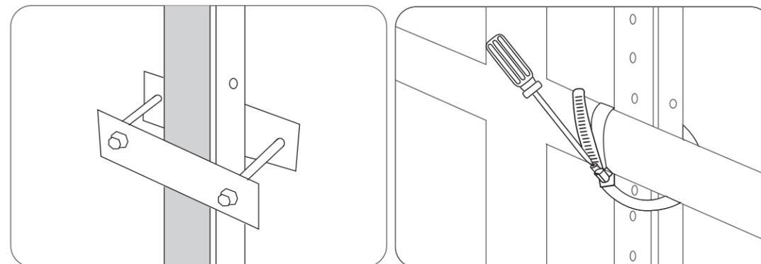
9. Install the microinverter to the balcony railing with stainless steel hose clamps.
