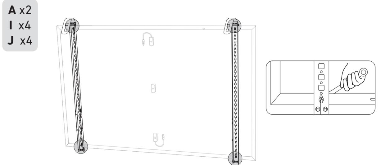
4. Tighten all the screws with 5N.m torque.
