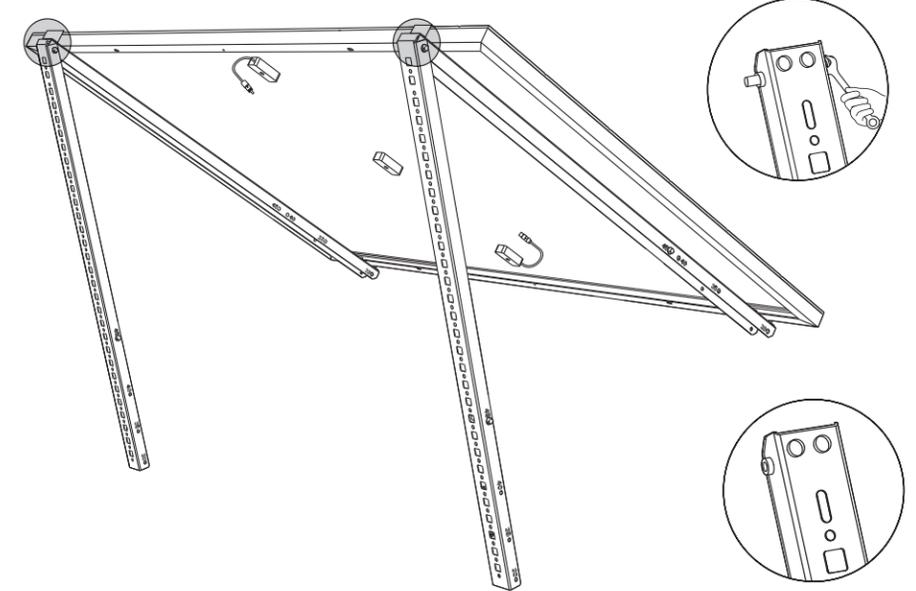
4. Mount the lower support beams and adjust the angle for maximum sunlight exposure.
