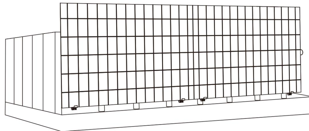
9. Connect the solar panel and the microinverter with the solar panel extension cables. When the LED indicator starts flashing, wait for 90 seconds.
