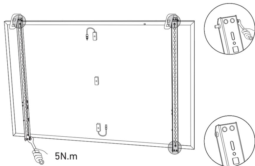
5. Connect the solar panel with the solar panel extension cable.
