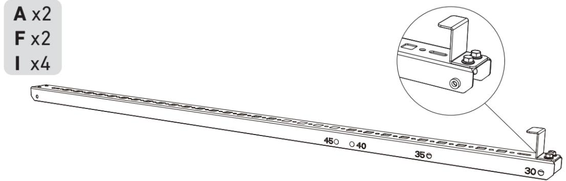
2. Place the silicone buffer pads onto the U-shaped racks, then mount the U-shaped racks to the solar panel's support beams.
