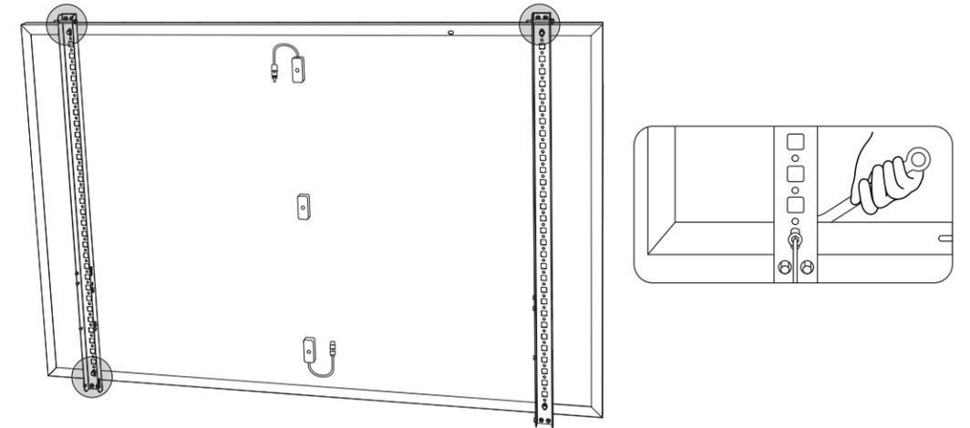
3. Install the vertical support scaffoldings and solar panel support beams without tightening the screws.
