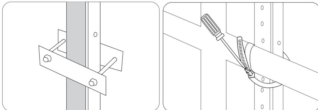
7. Install the microinverter to the balcony railing with stainless steel hose clamps.
