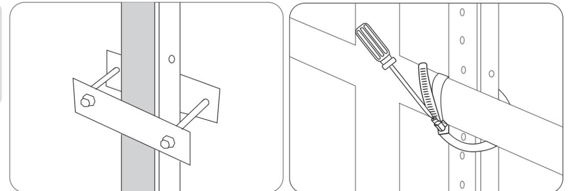
9. Install the microinverter to the balcony railing with stainless steel hose clamps.
