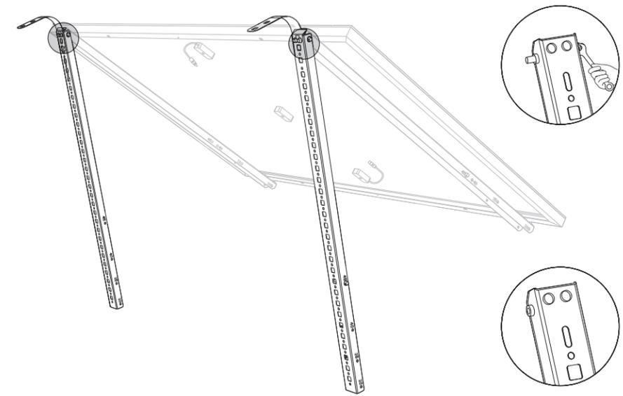
5. Mount the lower support beams and adjust the angle for maximum sunlight exposure.
