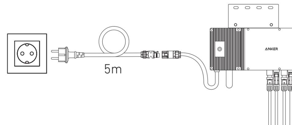
14. Download the app, and follow the in-app instructions to finish the microinverter configuration and Schuko cable connection.
