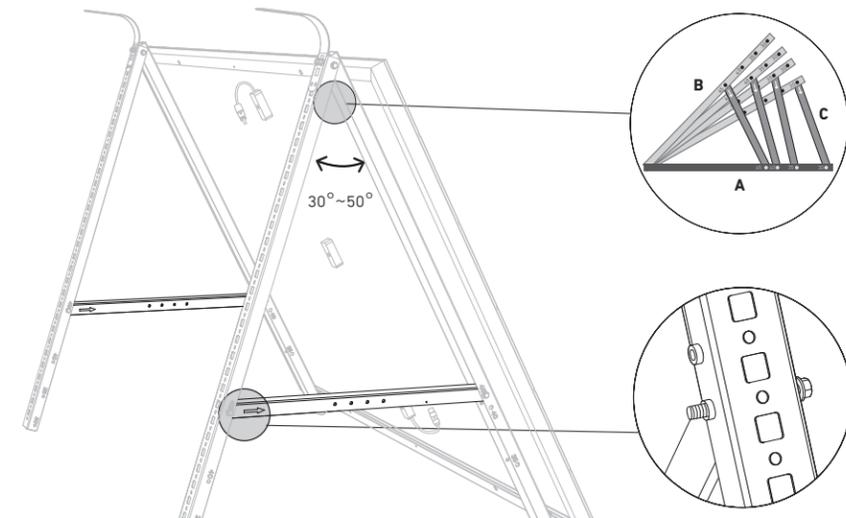
6. Tighten all the screws with 5N.m torque.
