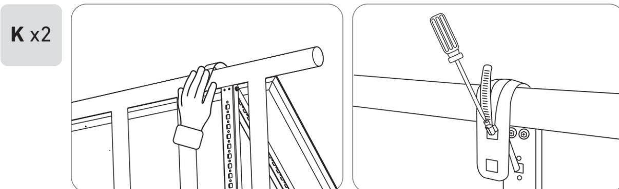
10. Install the solar panel's support brackets on the balcony railing, then secure them using fastening clamps and stainless steel hose clamps.
