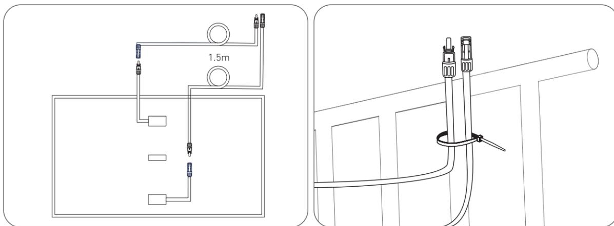
6. Fasten the Mounting Auxiliary Rope to the bracket and the balcony railing. Make sure the rope is tightened.
