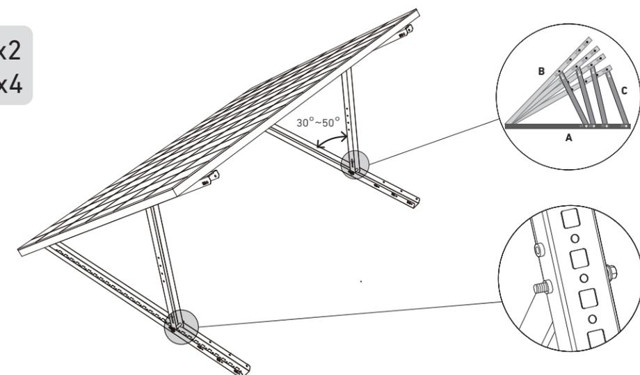
5. Align the solar panel with the holes on the vertical support scaffoldings to mark four mounting points. Mounting points on the same vertical support scaffolding should be 800mm (31.4in) apart.
