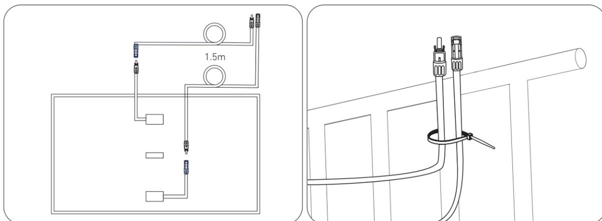
7. Fasten the Mounting Auxiliary Rope to the bracket and the balcony railing. Make sure the rope is tightened.
