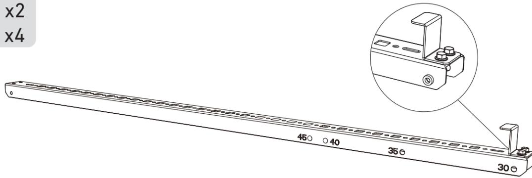
2. Place the silicone buffer pads onto the U-shaped racks, then mount the U-shaped racks to the vertical support scaffoldings.
