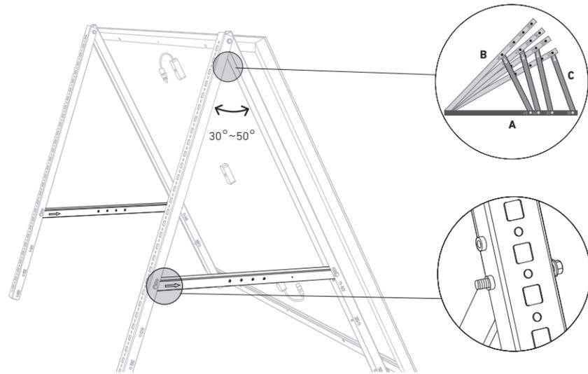
5. Tighten all the screws with 5N.m torque.
