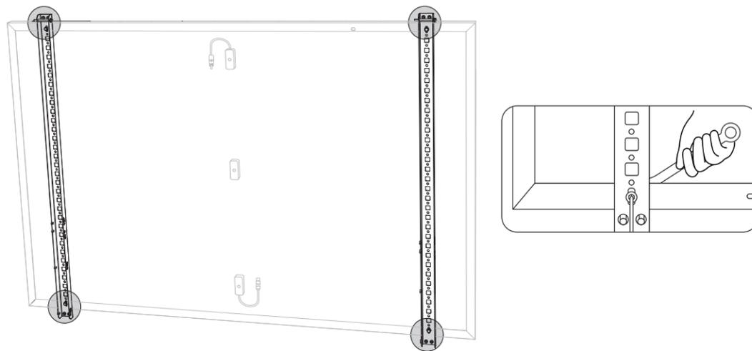
4. Install the vertical scaffolding and solar panel support beams without tightening the screws.
