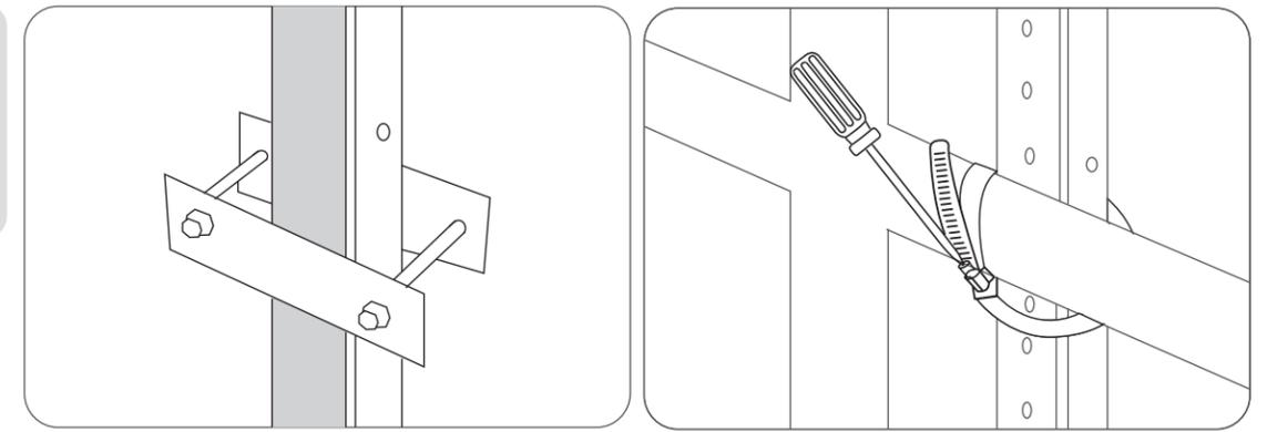
11. Install the microinverter to the balcony railing with stainless steel hose clamps.
