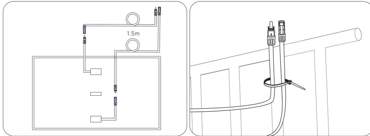
8. Fasten the Mounting Auxiliary Rope to the bracket and the balcony railing. Make sure the rope is tightened.
