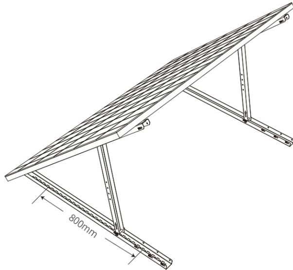
6. Remove the solar panel, mark the mounting points, and drill the holes 63mm (2.4in) deep with an electric drill. Then, secure the scaffolding with nuts.
