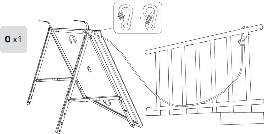
9. Hang the solar panel on the balcony railing and adjust the U-shaped racks manually to fit the shape of the balcony railing. Then, secure the U-shaped racks with stainless steel hose clamps.
