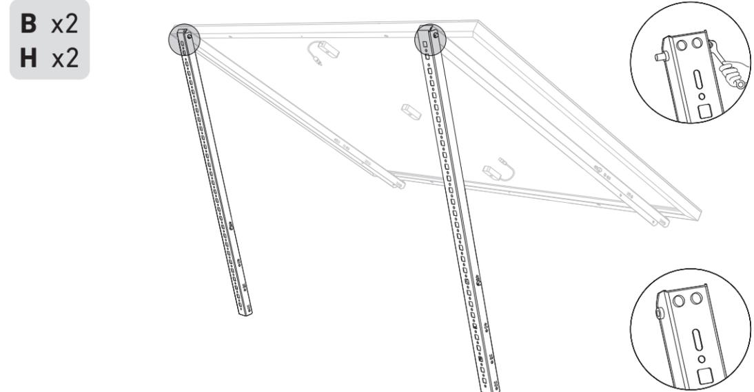
4. Mount the lower support beams and adjust the angle for maximum sunlight exposure.
