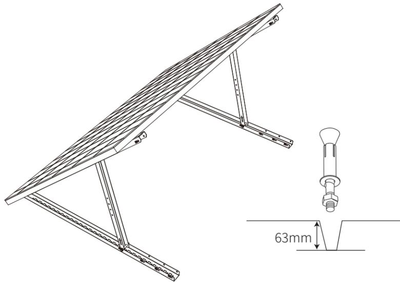
7. Tighten all the screws with 5N.m torque.
