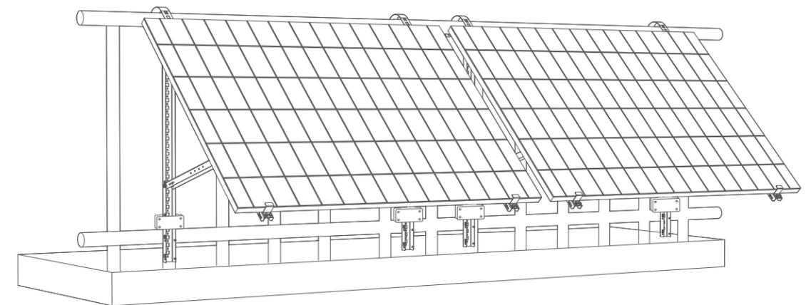
13. Connect the solar panel and the microinverter with the solar panel extension cables. When the LED indicator starts blinking, wait for 90 seconds.
