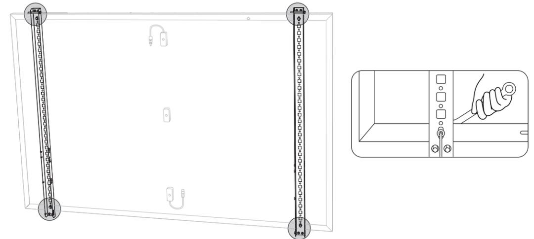
3. Tighten all the screws with 5N.m torque.
