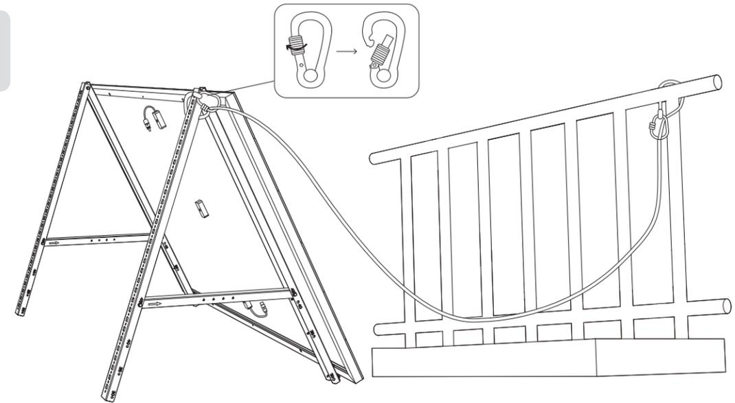
8. Install the solar panel's support brackets on the balcony railing, then secure them using fastening clamps and stainless steel hose clamps.
