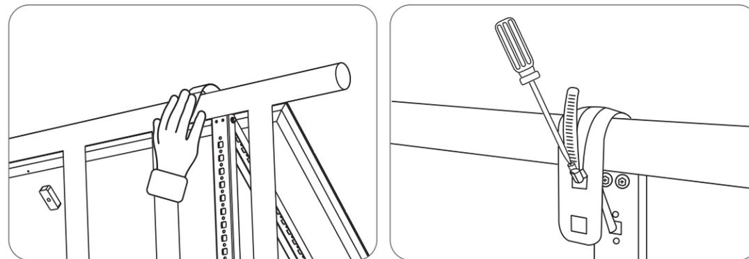
8. Install the solar panel's support brackets on the balcony railing, then secure them using fastening clamps and stainless steel hose clamps.
