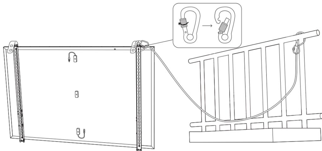
7. Hang the solar panel on the balcony railing and adjust the U-shaped racks manually to fit the shape of the balcony railing. Then, secure the U-shaped racks with stainless steel hose clamps.
