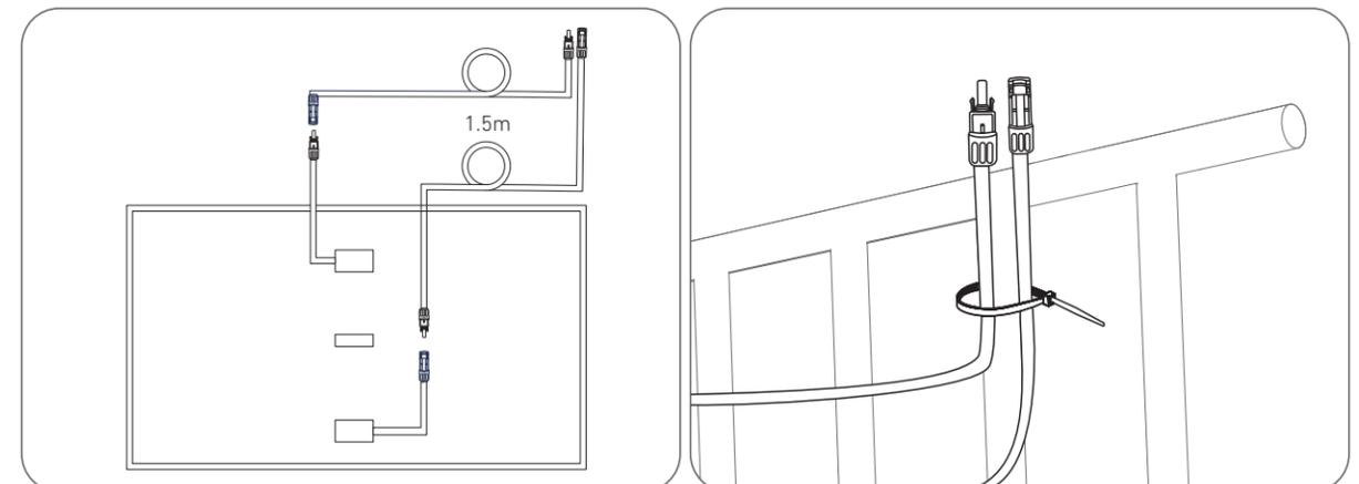
5. Fasten the Mounting Auxiliary Rope to the bracket and the balcony railing. Make sure the rope is tightened.
