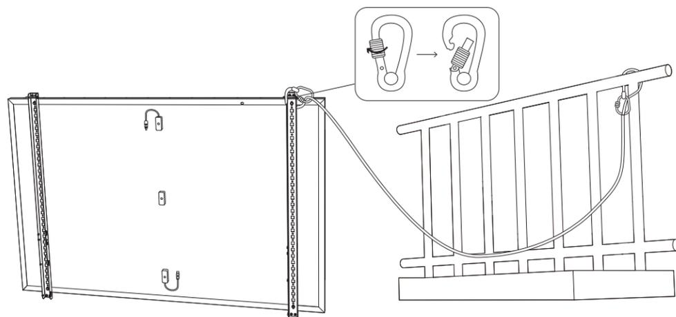
6. Install the solar panel's support brackets on the balcony railing, then secure them using fastening clamps and stainless steel hose clamps.
