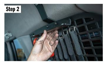
Now put the shelf mount in place. It sets on top of the other parts. Using the longer 1/4 bolts in your hardware kit, put a washer on and put the bolt in place. The mount goes with the long side pointing forward.
