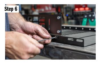
Next install the middle connector on one of the sides only. It doesn't matter which one. Again, put a washer on a bolt and thread them in place. Leave these bolts hand tight.
