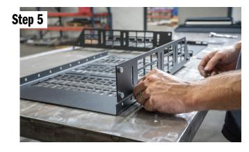
Install 3ea 1/4 bolts along the bottom of the back panel. Make sure to install a washer onto each bolt before installation. Do this on both shelve parts.
