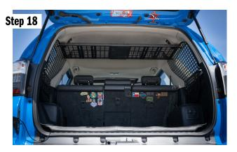
With everything in place, apply pressure to the center of the shelf causing the two shelf halves to become parallel. Then tighten the middle mount hardware. After that move your way around the shelf and tighten all the remaining bolts.
