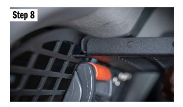
Starting with the side that does NOT have the middle mount, place the tabs of the shelf into the molle holes. The panel will need to be adjusted front to back and then when centered will pivot up and into place.
