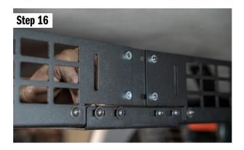
Now install the backing plate that connects the two back panels. Put in place and install 4ea bolts with washers.
