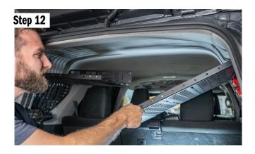
Similar to the previous step, slide your other molle shelf into the slots, center and pivot it up. This time the center mount will slide over the shelf on the other side. Push the shelf all the way into position, and install 4ea bolts with washers into the center mount connecting the two panels together.
