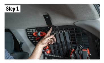
First we need to remove the 2ea bolts that holt the side molle panel to the top mount. Do this on both sides.
