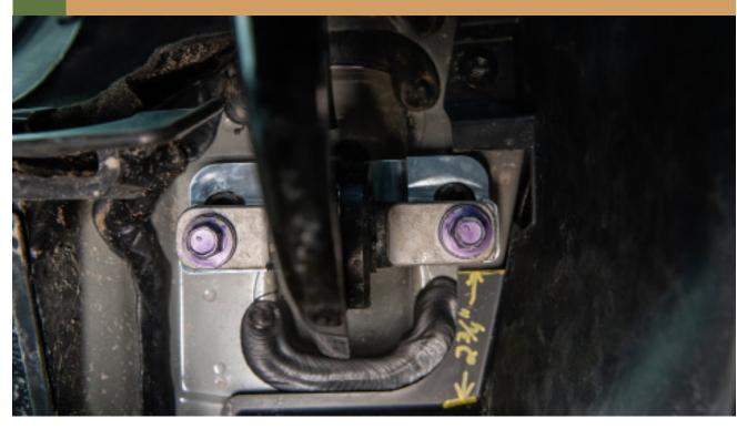
INSTALL SHOCK SPACER WITH SUPPLIED HARDWARE
