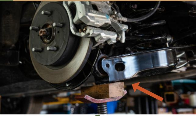
REMEMBER TO HAVE THE BOLT POINTED TO THE FRONT OF THE VEHICLE
