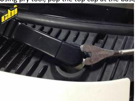
b. With the 12mm socket and tool driver of choice, remove the nut
