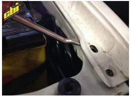
c. Lift fender piece at seam with your hands and pull back enough to access the bolts that hold the hood hinge down
