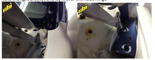
c. Use (2) 8mm bolts with (2) 3/8" washers and thread by hand into the holes
