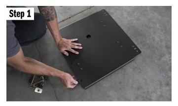
Grab your (4) slide on nuts. There are (4) holes at the edge of the skid. Slid the nuts onto the skid so that the flat side is on the flat side of the skid. If you push these too far over the hole, use your screw driver to help move them back and align them.
