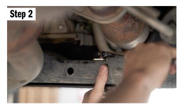
Using a 12mm socket, remove the (8) bolts that hold on the (2) bolt in supports.
