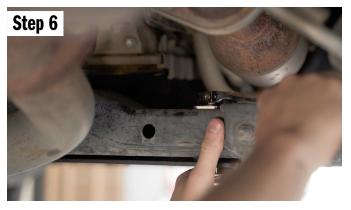
Grab your carriage bolt and from the bottom push it through the square hole in the skid, through the crossmember and the backing plate we previously installed. Then put on a washer and nut. Do not tighten anything at this time.
