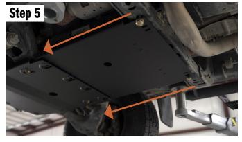
With the use of a floor jack or a friend, lift the skid in place. Set the front side of the skid with the clip on nuts, on top of your front skid. As a reminder you need to have the Cali Raised front skid in order to install the transmission skid.
