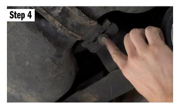
If you do NOT have TRD Tank Straps. Use a floor jack and put pressure on the gas tank to hold it in place. Remove the 12MM bolt holding the strap.
