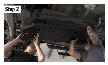
Using a floor jack or a friend, lift the skid plate into position and put the threaded studs though the (4) holes on the skid.
