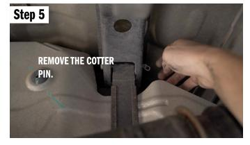
Then allow the strap to fall down. Remove the cotter pin on the other side, then remove the 1/4" pin that holds the strap in place.
