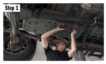
If you have a TRD Off-Road, remove the (4) nuts that hold on your factory gas tank skid with a 12mm socket. Remove the factory skid.
