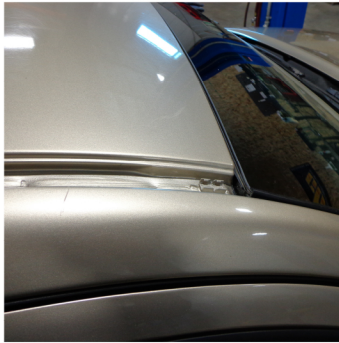
The weather stripping is held in place by the tabs shown above and pulls up
