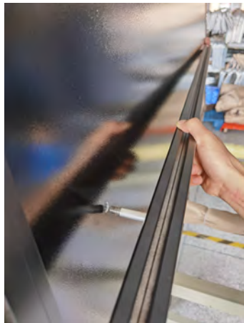
The mounting extrusion fitted to the base of the tent with the slide plate and bolt fitted.
