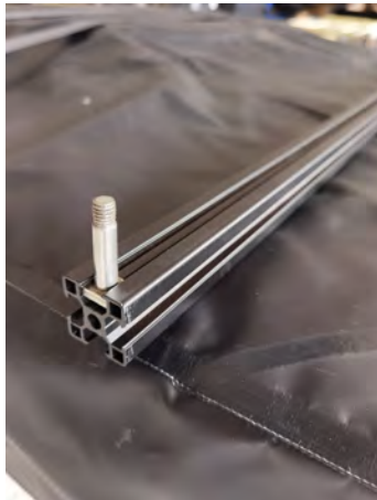
The mounting extrusion fitted to the base of the tent with the slide plate and bolt fitted.
