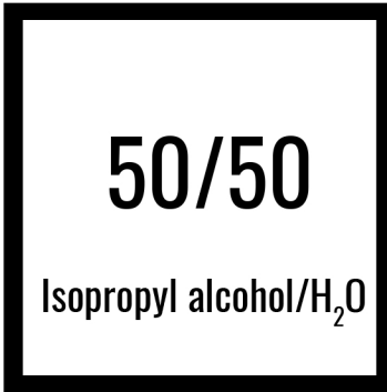
To prepare the surface for application of the front mounting foot clean the area on the roof of the vehicle with a 50/50 isopropyl alcohol/water mixture and allow to dry.
