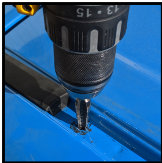
The furthest rear hole on each side will have to be drilled out to 3/8" to accept the plusnut
