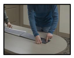
Line up the first set of holes and lighty press down only in the immediate area surounding and inbetween the holes.
