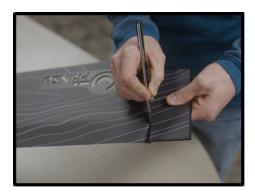
To trim out the area for the light bar cutout use the supplied knife. Begin from the top and cut down to the edge of the light bar cutout. Do this on both sides of the wind deflector.
