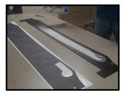
Clean the surface of the wind deflector to remove any dust and contaminates. Rubbing alcohol or any cleaner that doesn't leave residue behind can be used.
