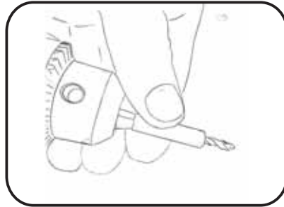
It is important to place tape around drill bit in order to stop the drill going too deep, the drill should only protrude a maximum of 10mm
