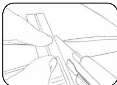
Use a straight edge to mark and cut rubber strip.
