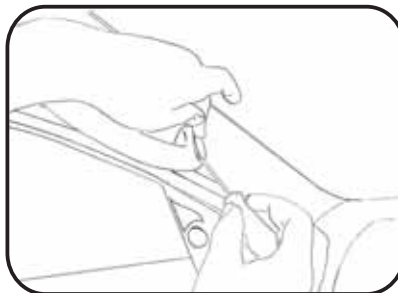
Pry plastic cover open with small flat screwdriver to gain access to bolts in handles.
