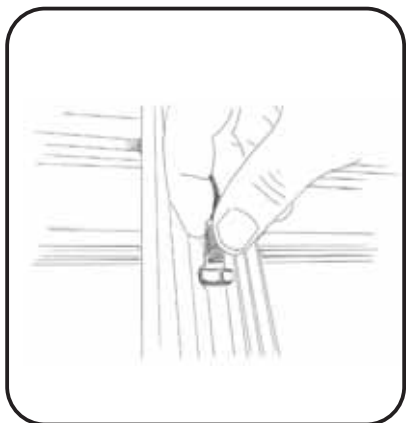
Remove rack from box, turn upside down, slot bolts into position onto slide rail.
