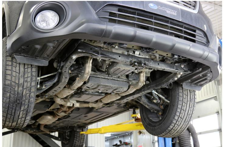
**#1 : Unscrew the bolt of the bumper beam.**
