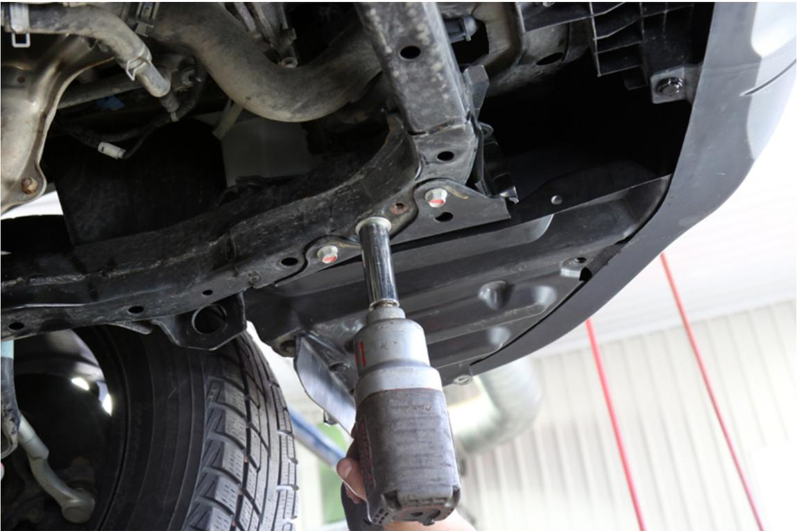
**#4 : Attach the bumper guard to the bracket,
