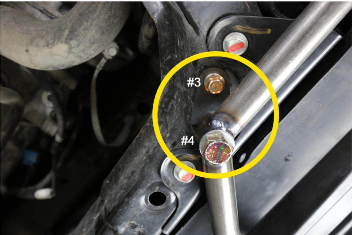
**#6 : You can now completely tighten the bolts of the bracket**
