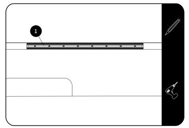
Position the Track (Item 1) against the side wall of the load bin, aligning the two center holes in the Track with the two 61mm markings made in 2.1.
