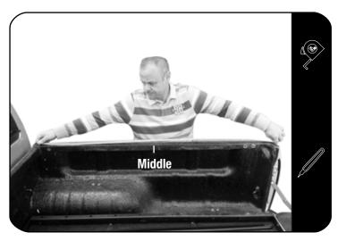
Measure the length of the load bin from the back of the cabin, below the rear window to the start of the tail gate.
