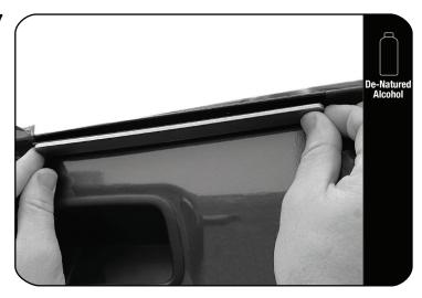
Clean the inside bottom edge lip using De-Natured Alcohol. Remove the backing tape from the self-adhesive tape on the Press Plate (Item 4) and firmly secure the Press Plate to the inside bottom edge lip as shown.
