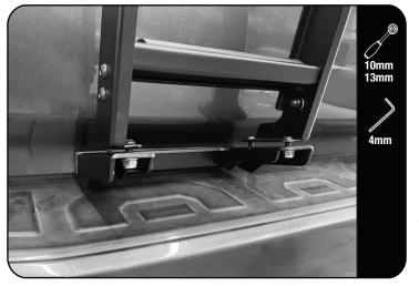
Hook the ladder over the studs in the Top Mount Bracket and lower the ladder. Loosely secure the ladder to the Bottom Bracket using four M6x16 Button Head Screws, four M6 Flat Washers and four M6 Nyloc Nuts (Item 5, 8 & 7).
