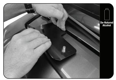
Clean the surface where the Top Mount Bracket (Item 19) wil be secured with De-Natured Alcohol.
