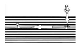
( C ) Position the Load Bay Legs as required and secure in position. Turn the Load Bars over so that the Bolts inserted in Step 2A are facing down. Lower the Load Bars onto the Legs, lining up the bolts in the Load Bars with the holes in the Legs. You may need to adjust the position of the Bolts.
