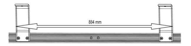
With your Rack in the upside down position ( Product Sticker should be upside down ) and working with the second Slat in, both front and rear, slide two M8 x 25 Hex Bolts supplied with the Universal Load Bed Legs into each end of the Slat using the machined Slots as shown.
