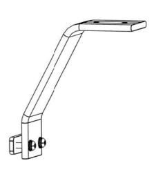
( **B** ) Slide two M8 x 25 Hex Bolts supplied with the Universal Load Bed Legs into each end of the Load Bars using the machined slots as shown.
