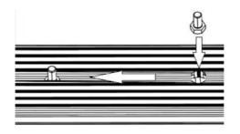
( **D** ) Grab your friend and with one of you on each side of the Rack, flip it end over end so that the bolts are facing down. Approach the vehicle from the rear lifting the Rack above the Legs. Slowly lower the Rack lining up the bolts in the Rack with the holes in the Legs. You may need to adjust the position of the Legs.
