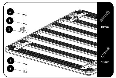
Loosely fit the Foot Top (Item 1) to the Between Slat Foot Adapters using M8 x 16 Hex Bolts, M8 x 16 x 1.6SS Flat Washers and M8 Nyloc Nuts (Items 4, 5 & 6) as shown.
