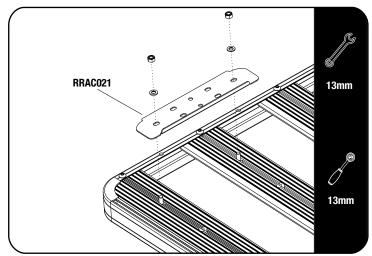
**Loosely fit two pairs of Between Slat Foot** Adapters - RRAC021 (supplied with KRS0002T) to the bottom of the Slimline II Rack.
