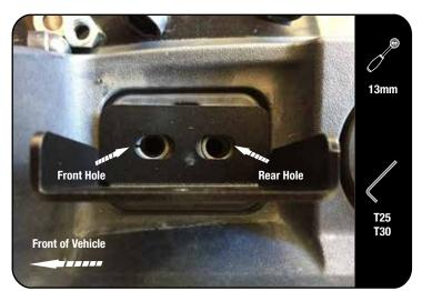
Remove the bolts of the OEM crossbars and the four tie-down plates.
