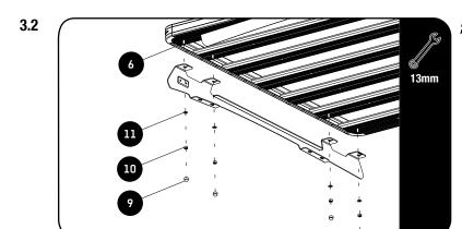
Fit your Roof Rack to the Foot Rails using M8x20 Hex Bolts, M8x16x1.6SS Flat Washers and M8 Nyloc Nuts (Items 6, 11 & 10) as
