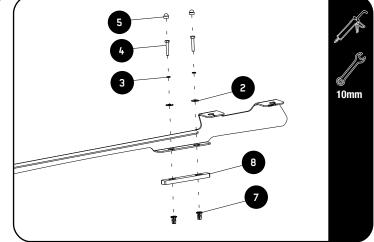
Place a bead of silicone around each of the Jack Nut openings inserted earlier in Step 2.5.
