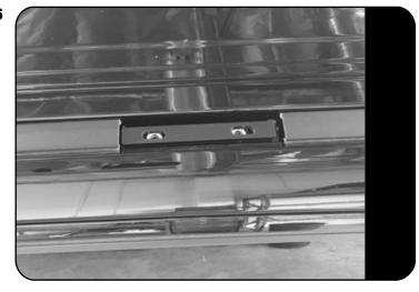
Place the four Spacers (Item 8) back on top of the inserted Jack Nuts in 2.5. Fit the three pieces of the ditch moulding cut in 2.3. With the ditch moulding in place, remove the Spacers.
