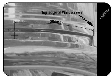
Mark the middle of the ditch by measuring 390mm from the top edge of the windscreen.
