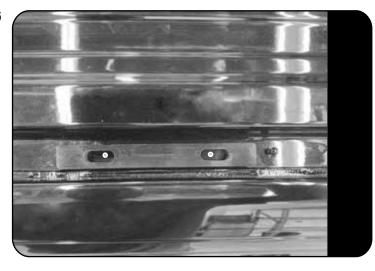
Verify that the markings line up with the slots in the Spacers (Item 8) before drilling the mounting holes.
