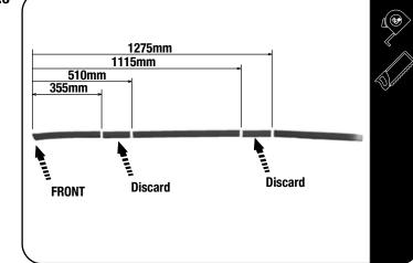
Lay the righthand ditch moulding on an even surface. From the front tip of the ditch moulding, measure and mark as shown.
