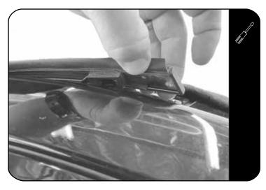
Using a flat screw driver and starting from the front of the vehicle, lift and remove the two ditch moldings running along either side of the roof.
