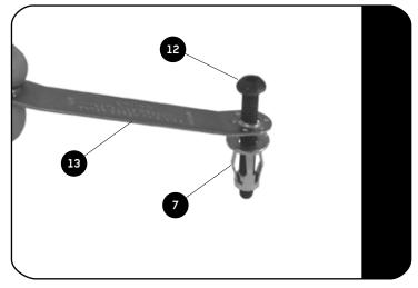
Insert the M6 Button Head Bolt (Item 12) into the one side of the Jack Nut Tool (Item 13). Loosely fit a Jack Nut (Item 7) to the Button Head Bolt as shown. Using the Jack Nut Tool and a M6 x 30 Button Head Bolt, insert the M6 Jack Nuts into all 8 holes. Place the assembly into the hole drilled. Using a Battery Powered Screw Driver and a H4 Allen Key Bit, set the Jack Nut into the hole while holding onto the handle of the Jack Nut Tool.
