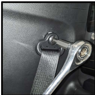
Moving to the C pillar remove the seat belt
