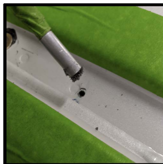
Do not expand the holes in the front closest to the windshield
