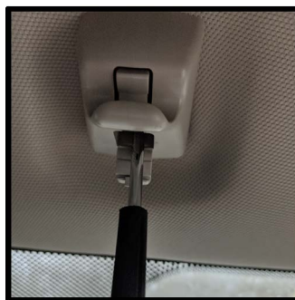
Next remove the sunvisor hangers ...
