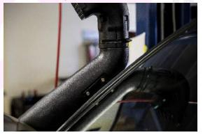
17. Mark the top Mounting bracket by marking the inside edge with a pen and the top and bottom edges.
