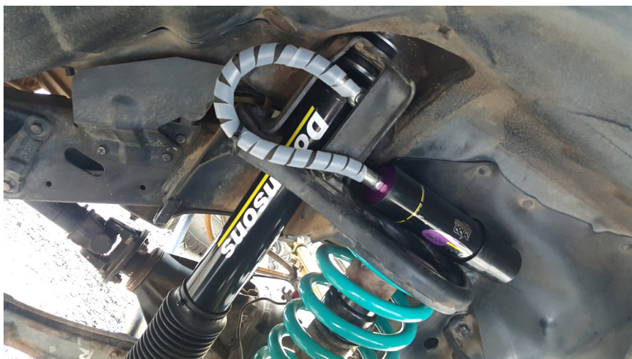
Nissan Patrol GQ/GU - Y60/Y61 Mounted to existing coil tower cover plate bolts with longer bolts supplied
