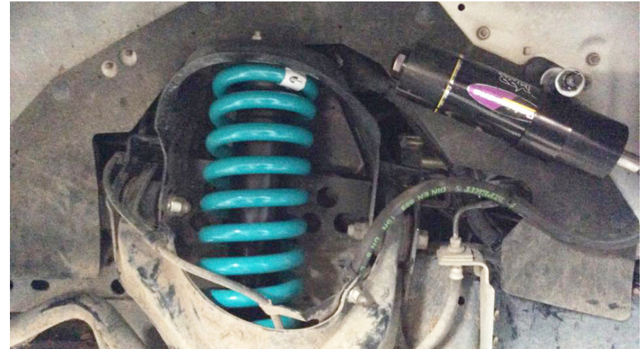
Toyota Hilux 2012 Mounted through the chassis rail
