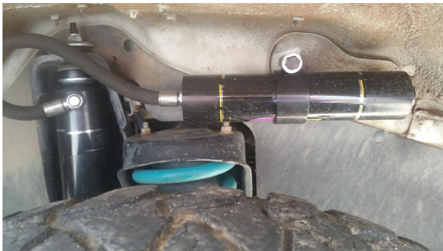
Nissan Patrol GQ/GU - Y60/Y61 Mounted to existing coil tower cover plate bolts with longer bolts supplied
