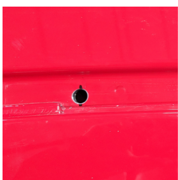
Drill one hole on both sides of the truck. The recommended hole size from plus nut is .386"-.391"*
