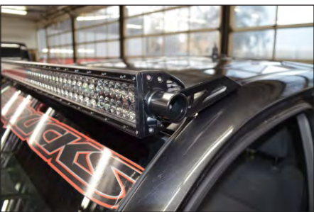
STEP 13 - Route power wire down A-pillar. Apply a small bead of silicone and tape wire down allowing silicone to set. Wire light bar according to additional instructions supplied with KC light bar.
