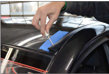
STEP 1 - Tape off truck to protect paint from scratches. Lift up rain gutter molding in front corner.
