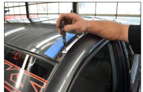
STEP 6 - Mark front hole with center punch. Double cab trucks use factory rear Nut-Certs already installed. Access cab trucks will require marking the rear hole and will not use the center hole.
