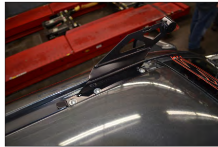
STEP 11 - Install driver side bracket with supplied hardware. Install other bracket onto KC light bar.
