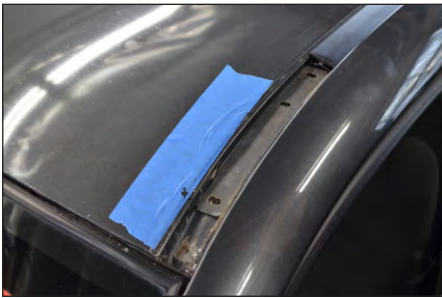
STEP 10 - Place rubber gasket in gutter. TIP - (Customers in extreme climates can add silicone to gasket to prevent leakage possibilities)
