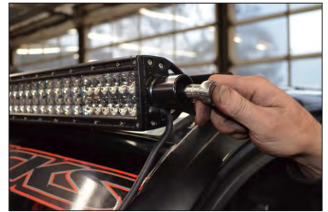
STEP 12 - Install KC light bar into driver side bracket and drop passenger side down onto truck. Bolt KC light bar on and fasten bracket down on passenger side.
