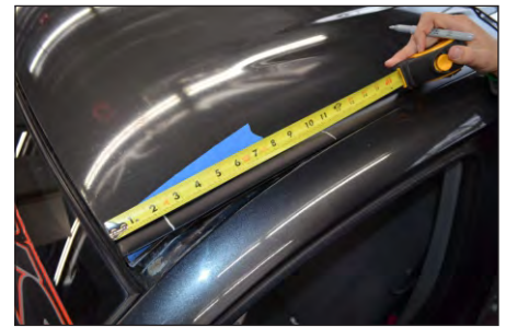
STEP 3 - From the front windshield edge of molding, measure out 2.5" and 10.75" and make a mark.
