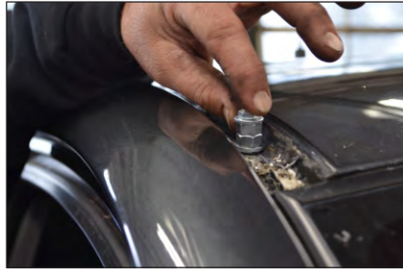
STEP 8 - Insert supplied Grip-Sert into the holes. (Small amount of silicone on splined area is recommended)
