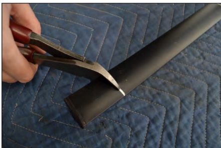
STEP 4 - Cut rubber molding on marks and remove center. Re-install front and rear molding pieces.
