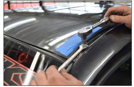
STEP 9 - Use tool to fasten Grip-Sert by tightening down the bolt while placing wrench on center nuts. DO NOT let Grip-Sert turn when tightening.
