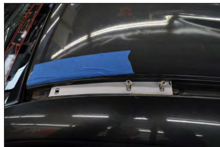
STEP 5 - Cut out template and lay in gutter with back edge 10.75" from edge of windshield.
