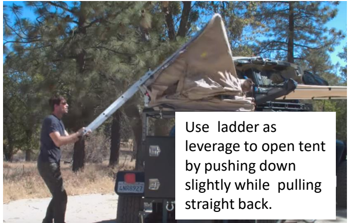
Fully extend ladder. Excessive force will damage tent base/floor.
