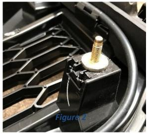
NOTE: Removal of the studs can be completed by holding the flat or built-in washer portion of the stud with Channellock pliers, while backing the nut off with a 10mm socket or wrench. Make sure not to damage the threads on the studs.
