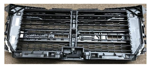
7. Separate the two sections of the grille and lay the inner-grille down, with the front facing upward.
