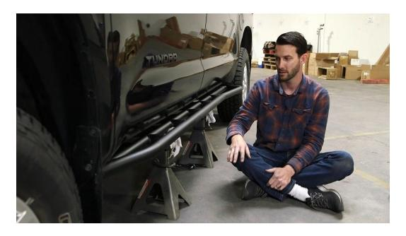
For this step, you'll need to have 2 jack stands. You'll then position them inside the wheel wells, and place the slider on top. Be sure to put a cloth between the slider and each jack stand, this will ensure the powder coating doesn't scratch.
