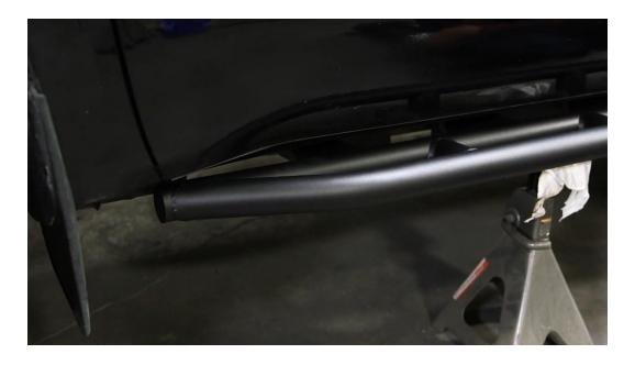
Make sure the slider is centered inside the wheel wells, there should be about 3" on each side between the end of it and each mud flap.
