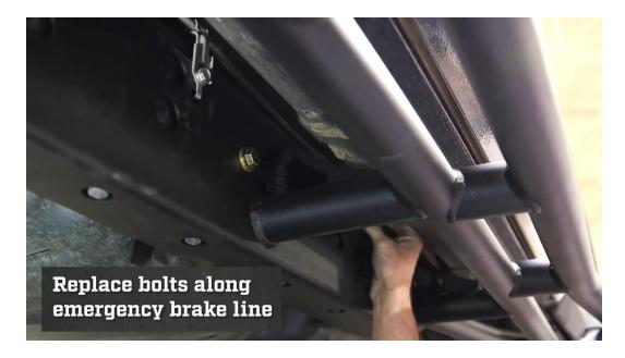
Remember those brackets we moved out of the way earlier for the emergency brake line? Go ahead and put each of those back in place.
