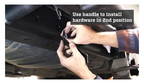
On the driver side, though, is the gas tank, so for that one, you'll have to use the included handles to reach the backside of the bolts. To do so, insert a square nut into the handle, and use it position it into place.
