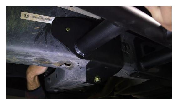
For this one, you'll grab a large bolt, add a washer and a backing plate, and insert it through the inside hole, where it will come out through the slider. Add another washer and locknut, and hand-tighten it.
