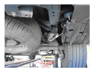
Complete the assembly by loosely attaching the Tailpipe Assembly to the Mid-Pipe using a supplied 2.50" clamp and inserting the hanger into the rubber insulator.
