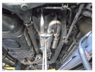
**Step 3:** Next attach the Oval Muffler to the Inlet Pipe with the supplied 2.50" clamp. This exhaust system is configured to allow the user to tune the sound. For a more moderate exhaust tone install the U-pipe Assy and the 4.00" NDT (No Drone Technology) Chamber (as shown) using the suppled 2.50" clamps. For a more aggressive sound see configuration chart below.
