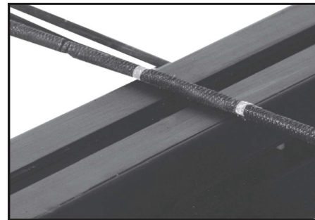
13. Mark your string to ensure that you are cocking the bow in a consistent manner. Due to the high draw weight involved in cocking the bow, it is easy to cock the crossbow off center. Failure to cock the crossbow squarely will result in poor accuracy. Simply mark the string with a marker or other means visibly ensure the bow is being cocked properly.
