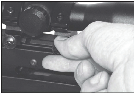
12. Tighten the locking nuts by hand or with a screw driver if needed.
