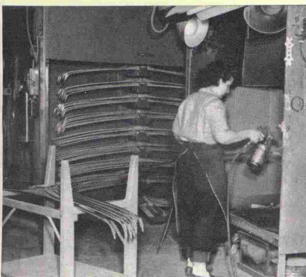
For that characteristic Bear custom finish archers admire, each bow has several hand-rubbed coats of durable varnish.
