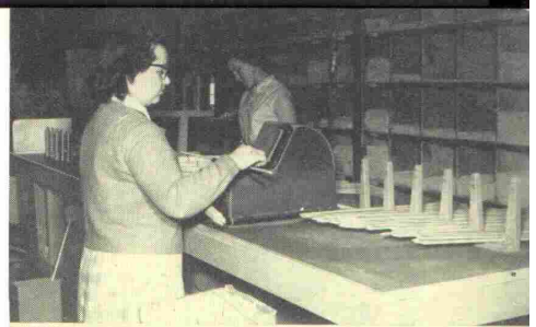
Selecting, weighing and classifying arrow shafts with aid of shadowgraph scale.
