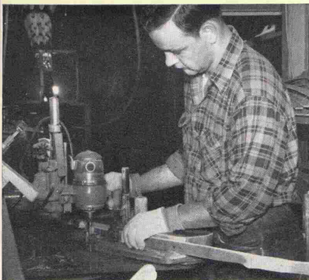
All the way through, human skill and precision machine work toward perfection. This high-speed router shapes recurve bow tips.
