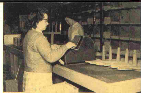
Selecting, weighing and classifying arrow shafts with aid of shadowgraph scale.
