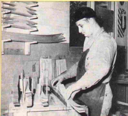
5. Sub-assembling component parts of a Bear Bow — wood core pieces, Fiberglas face-and-backing strips and handle section.
