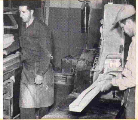
3. Sanding each piece of bow core stock and Fiberglas to exact size and uniform thickness insures uniformly accurate shooting.
