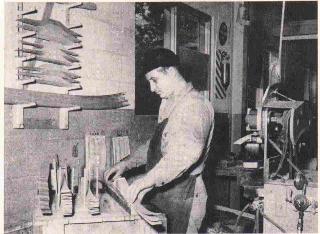
Sub-assembling component parts of a Bear glass-powered Bow—wood core pieces, Fiberglas face-and-backing strips and handle section. Each piece must first pass rigid inspection.
