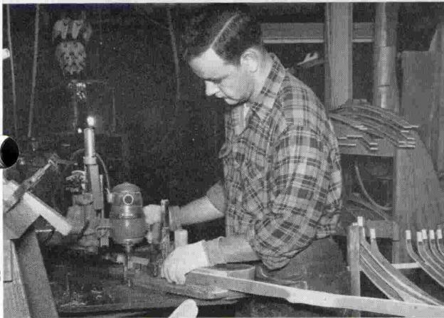
All the way through, human skill and precision machine work toward perfection. This high-speed router shapes recurve bow tips.
