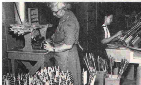
With glowing wire, feathers are trimmed to final shape.
