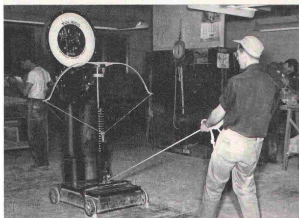
On this new model specially-equipped scale—most accurate of its kind in the U.S.—every Bear Bow is "weighed" for draw weight.
