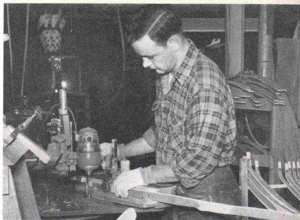
All the way through, human skill and precision machine work toward perfection. This high-speed router shapes recurve bow tips.
