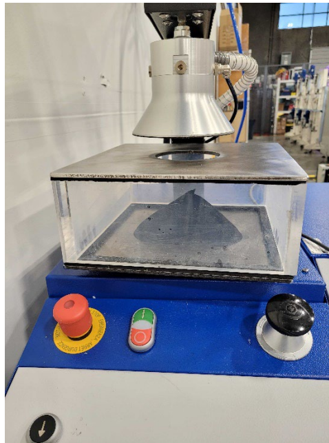
Figure 1. Black CAN95e Respirator under test using a TSI® CERTITEST® Automated Filter Tester Model 8130A.
