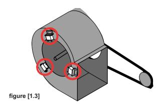
If using multiple ion generators, tie the wires of each generator together after mounting (if using the mounting plate, mount the generators to the plate and tie the wires of each generator together before mounting each plate). Be sure to keep all wires away from the generator tips, moving objects and areas that may cause wires to be sucked into the blower.
