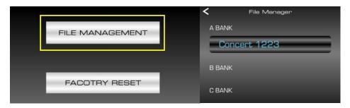
"FACTORY RESET" – Erases all the data in OC10W and restores the unit to factory default settings. Click the bar, then go to the device, use UP/DOWN button to choose "Y", then press ENTER button to start the reset.
