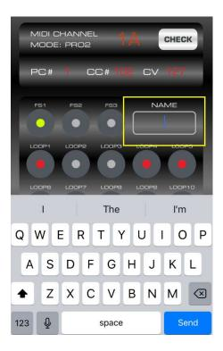
Scroll up/down a MIDI channel - edit PC# and CC#, check the validity by pressing the "CHECK' button, the MIDI output jack will send PC# and CC# once when pressed. In PRO1 mode, the MIDI channel 1 contains group 1A and 1B, MIDI channel 2 contains 2A+2B, etc. In PRO 2 mode, the MIDI channel 1 contain 1A, 1B, 1C, 1D, channel 2 contains 2A, 2B, 2C, 2D, etc.
