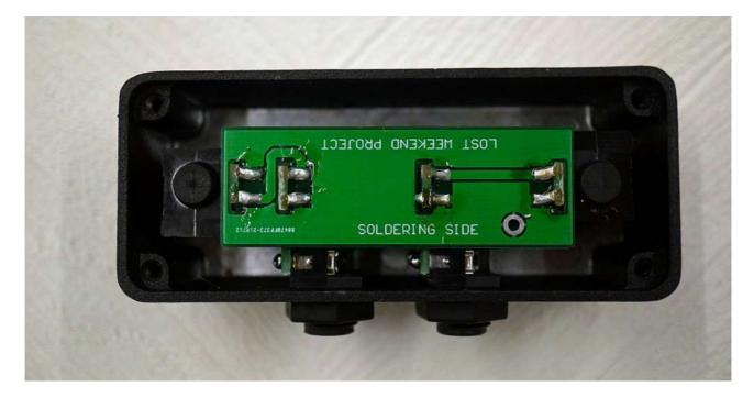
\*If the amount of solder is small, the power may not be applied properly. In particular, apply solder to the extent that the solder penetrates into the eyelet of the jack side board.
