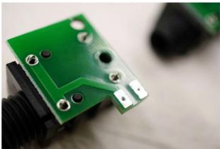
In this way, align the protrusion of the jack with the hole on the board and install it. This is a side PCB.
