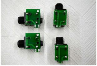
Once installed, solder the four terminals on each jack.
