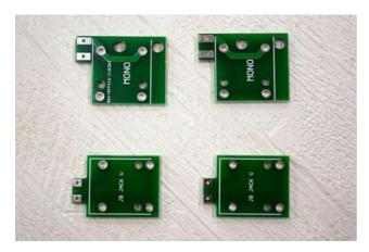
Attach the PCB for the jack to the jack. Attach the jack to the side with the letters on the board.
