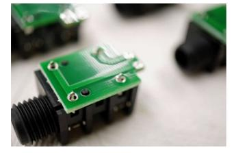
Attach the top jack PCB in the same way, aligning the jack protrusion with the board hole.
