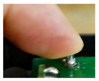
After applying the solder, check that the bar moves. If the bar moves when you press it with your fingers from above, there is no problem.
