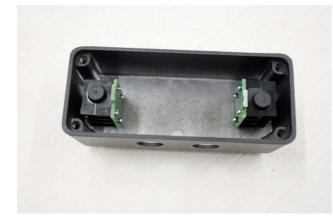
First, assemble the top side jack into the case. At this time, install the board so that it faces inward.
