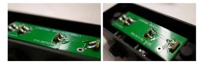
At this point, verify that the top and side terminals each have power. It's a bit noisy as the back is left open and there's no case shielding, but that's fine at this point.
