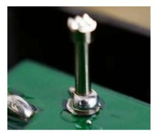
Solder the ground bar. At this time, do not apply solder to the silver bar.
