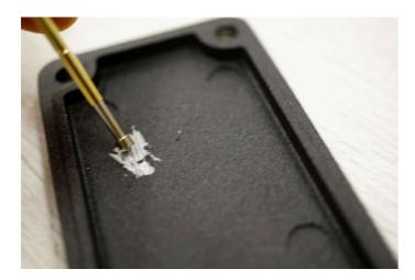
Slightly peel off the paint on the back cover where the ground bar touches.
