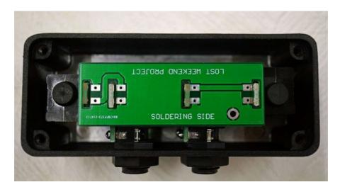
⑤ Fine-tune the angle of the four jacks so that the protrusions on the board fit into the holes in the main PCB. Adjust until it goes all the way in.
