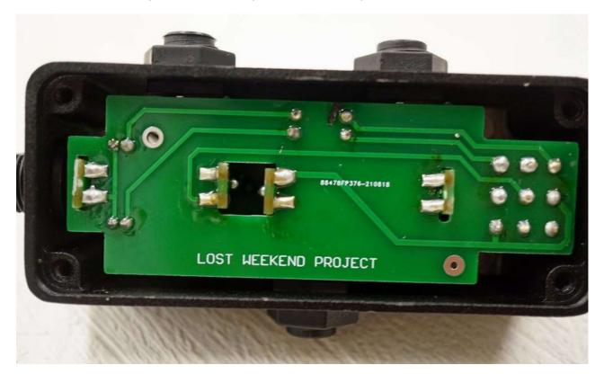
\*If there is not enough solder on the parts that are fixed at right angles between the jack PCB and the main PCB, the power may not be applied properly.
