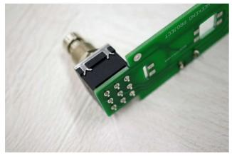
Insert the footswitch into the PCB hole. The foot switch has a certain orientation, but insert it in the direction that the foot switch lug fits into the hole in the PCB.
