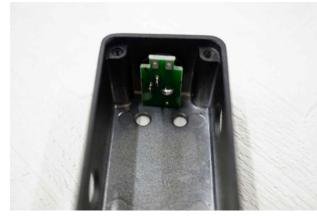
First, assemble the DC input terminal into the housing. Secure the DC input terminal by passing one washer under the nut. Next, install the three monaural jacks. At this time, install each PCB so that the protruding part faces upward.
