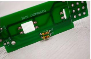
First, place the two resistors on the PCB where it says 4.7K. It doesn't matter which direction. The two resistors are both 4.7K, so they can be placed on either side.
