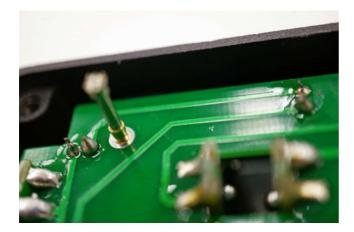
◄ First, thread the ground bar through the hole in the main PCB. Pass the bar until it touches the top of the case, and at that point make sure that the gold part of the bar is sticking out from the PCB.
