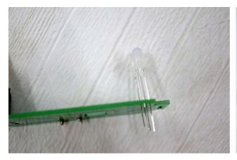
Two LEDs inserted. Do not solder the LED until the end. **That means no soldering at this point.** However, the LED may come off and fall while you are working on it.
