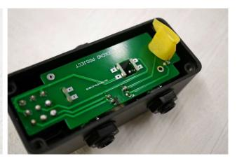
Once the main PCB is placed on it, adjust the protrusions on the PCB of each jack so that they fit into the holes in the main PCB.
