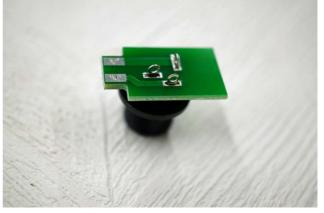
Now, install the DC jack and DC jack PCB. Similarly, attach the side marked with () to the board according to the correct shape of the terminal.
