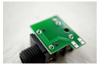
In this way, align the protrusion of the jack with the hole on the board and install it.
