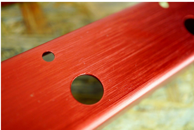
Perform grounding on the housing. First, remove the paint around the foot switch hole.
