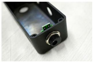
Secure the DC input jack with the washer and nut.
