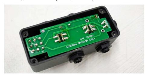
\*If there is not enough solder on the parts that are fixed at right angles between the jack PCB and the main PCB, the power may not be applied properly.
