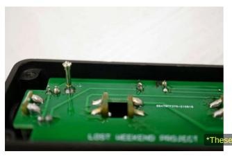
Solder the ground bar. At this time, do not apply solder to the silver bar.
