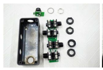
Temporarily assemble into the casing. Incorporate the jacks and the DC jack.
