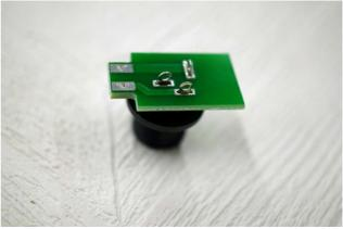
Now, install the DC jack and DC jack PCB. Similarly, attach the side marked with  $\bigcirc$  to the board according to the correct shape of the terminal.
