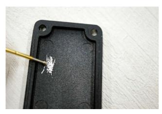
■ Slightly peel off the paint on the back cover where the ground bar touches.
