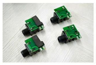
Paste it below the protrusion on the board like this. This is to prevent the jack boards from touching each other internally and causing electricity to not flow.
