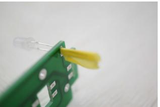
To prevent the LED from falling, use masking tape to secure the LED lead wires below the board to make the work easier. This step itself does not have to be performed. Be careful not to bend the lead wires by applying too much masking tape.
