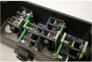
Once you're sure all four jacks and the board are well isolated, it's time to mount the main PCB.
