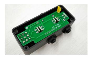
◆ Attach each jack by adjusting its position so that the protrusions fit securely into the holes on the main PCB.
