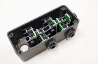
Next install the phone jack. Insert the jack to which the insulator was pasted earlier on one jack in each of the upper and lower tiers.
