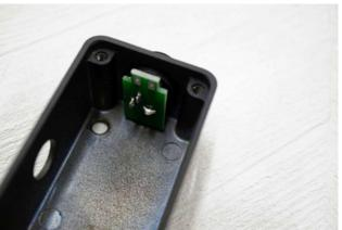
First, assemble the DC input terminal into the housing. Secure the DC input terminal by passing one washer under the nut. Next, install the three monaural jacks. At this time, install each PCB so that the protruding part faces upward.
