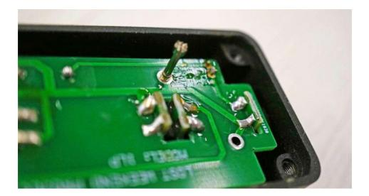
First, thread the ground bar through the hole in the main PCB. Pass the bar until it touches the top of the case, and at that point make sure that the gold part of the bar is sticking out from the PCB.
