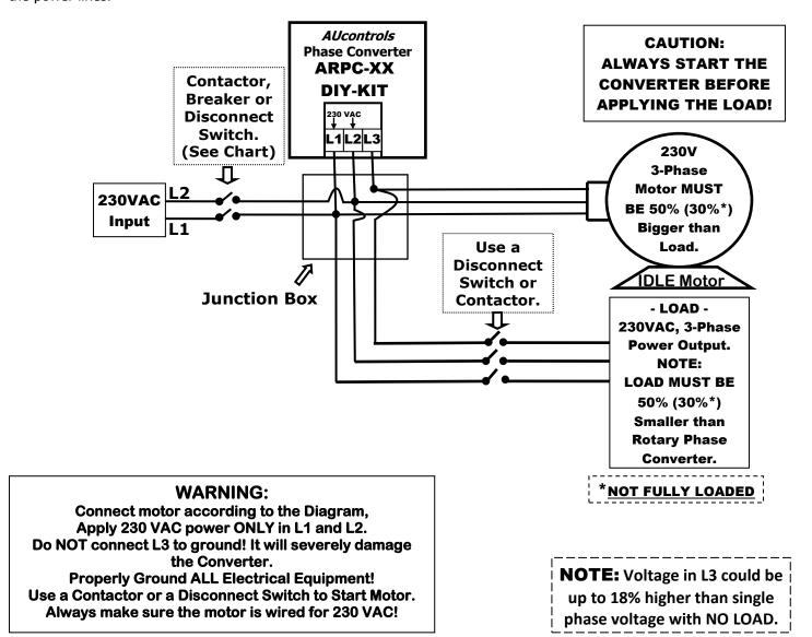
**3-Phase Rotary Motor MUST start within 5 seconds maximum**, if motor fails to start or it hums **turn power OFF** and check the wiring and/or the motor's bearings.
