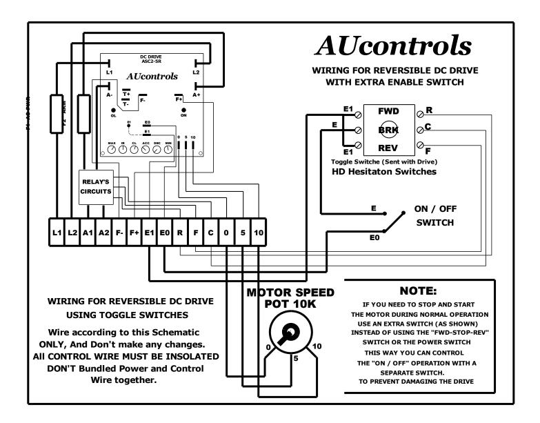
The Schematic shows the wiring to use an EXTRA switch to control STOP/START operation, NOT USING the "FWD-STOP-REV" switch provided with the Drive, this way you can leave the switch on FORWARD or REVERSE Position and just use the ENABLE SWITCH to STOP or to START the Motor.
