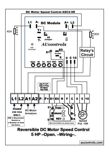
The DC Motor Speed Controllers **ASC2-5R** are **REVERSIBLE** which allows the motor to run Forward or Reverse.
