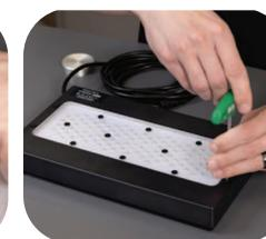
11. Replace the Radion cover and cover screws. **Important:** Do not overtighten.
