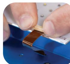
7. Place the new G6 cluster so that the screw holes line up, and the cluster pin holes connect to the driver board (being careful not to bend the pins). Make sure the cluster sits flush to the driver board, then re-insert the UI Ribbon as shown above. (ribbon contacts facing downward)
