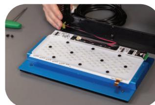
10. Place the **NEW** lens screws and hand tighten. **Important:** Do not overtighten.
