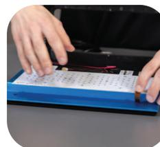
4. Remove the lens and cluster retaining screws. (T10 Torx Bit Required) Then remove the Lens. (You will not be re-using this lens) (10 screws for XR30) (6 screws for XR15)
