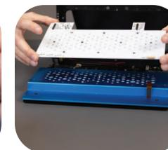
5. Carefully disconnect the cluster from the driver board and UI Ribbon and remove the cluster – the XR15 has x2 extra T10's holding the cluster to the pre-driver (these need to be removed) and the fan wire must be slid off of the cluster.
