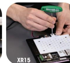
8. \*For the XR15 – ensure that the fan wire is routed back into place on the G6 cluster and the x2 extra T10 screws are secured holding the pre-driver to the cluster.\*
