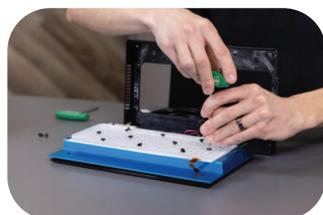
9. Carefully place the **NEW** lens. Important: Be gentle when placing the lens so as not to damage the LEDs. **DO NOT REUSE THE ORIGINAL LED LENS.**
