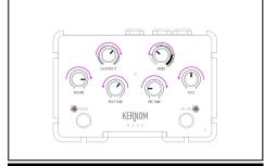
Repeat steps 2 and 3 on as many knobs as you like. If the user repeats the steps on all 6 knobs, the pedal leaves the preset as all knobs are now active.
