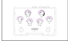
Repeat steps 2 and 3 on as many knobs as you like. If the user repeats the steps on all 6 knobs, the pedal leaves the preset as all knobs are now active.
