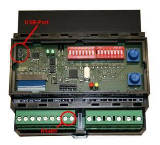
The left 3 DIP switches for the mode must be set to OFF, OFF, ON.
