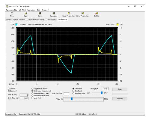
With the oscilloscope function, the channel selected on the left (dimmer 1 or 2) can easily be checked with different measuring methods. This allows the load to be checked for excessive current peaks, especially when retrofit lamps are in operation.
