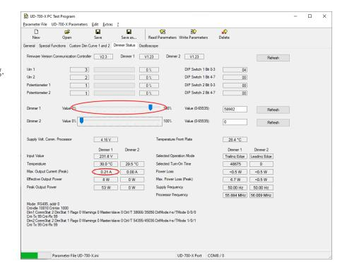
Now the inrush peak current is checked. Here select "Measurement on Start" and e.g. "Half Period No. 2" (if necessary also carry out tests with other settings). Setting "Dimmer 1", slider to the left, click "Measure" button, now pull up slider slightly. Here you can see that the peak current is 0.4 A.
