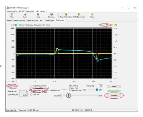
Countercheck in leading-edge phase control mode: On the "General" page, select "Leading Edge" on the right under "Default Operaition Mode" and click on "Write Parameters" at the top.
