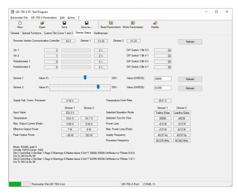
On the status page you can see information about firmware, analog inputs, potentiometers, DIP switches, voltages, currents and powers. In addition, the two dimming channels can be operated with the sliding potentiometers.
